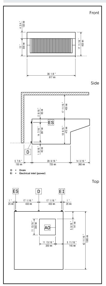
Ventilation Equipment Condensation hood with fan for 20 GN 1/1 electric oven
